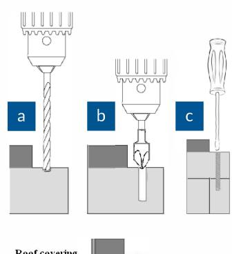
Measure out your fixing points on your kerb Panoroof recommend a fixing every 400mm, drill and countersink your fixing points.
