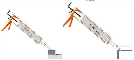
Position the Panotrade skylight glazing into the easy fit kerb (Please note: depending on the size you have purchased, this may require up to six people on site) ensuring the step of the glazing is set inside the rebate of the easy fit kerb
