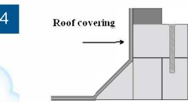
Now proceed to finish your roof covering up to the top of your easy fit kerb to fully encapsulate the kerb and joist / upstand.
