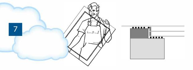
Apply pressure on the Panotrade skylight glazing to ensure an even spread of the silicone closing up any gaps and pushing out any air bubbles as you work your way around the perimeter of the rooflight. You should now have a impermeable bond between the easy fit kerb and the skylight glazing.
