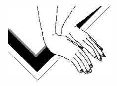
Leave the silicone to cure and then clean any excess off with a blade or scraper being carful not to scratch or mark your skylight glazing.
